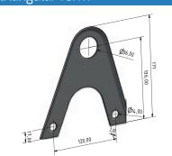
Suitable for 2 pipes with 32 mm  $\emptyset$  - The stacking element is mounted on the snow retention clamp (not included in the article) - PU 50 pcs
