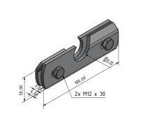
Snow retention clamp for standing seam and angle seam roofs, suitable for tubes with 32 mm Ø • Material of the clamp is selectable, srews out of stainless steel V2A 1.4301 • PU 10 pcs
