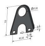
For tube fixation • suitable for 2 tubes with 32 mm  $\emptyset$  • mounted on the seam of the snow retention clamp (not included in the article) • PU 30 pcs
