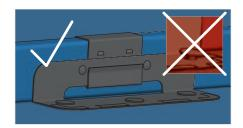
we recommend using the Fixed Clip Plus with countersunk holes.
